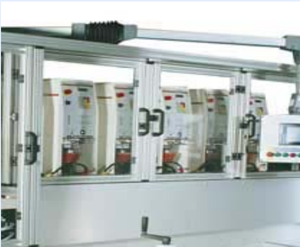
6 Colors Pad Printing System for plastic cosmetics with approx. 2000 rollers/hr
