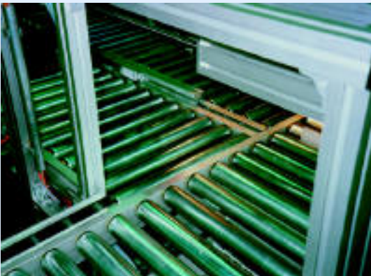
Roller conveyor transfer with steel rollers in distribution center.
