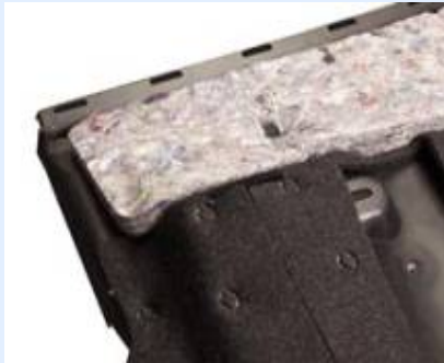
Riveting of insulation material on plastic automotive part
