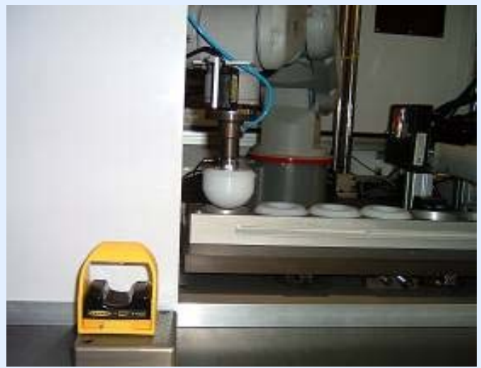
Robot with part present sensor for automatic Pick and Place
