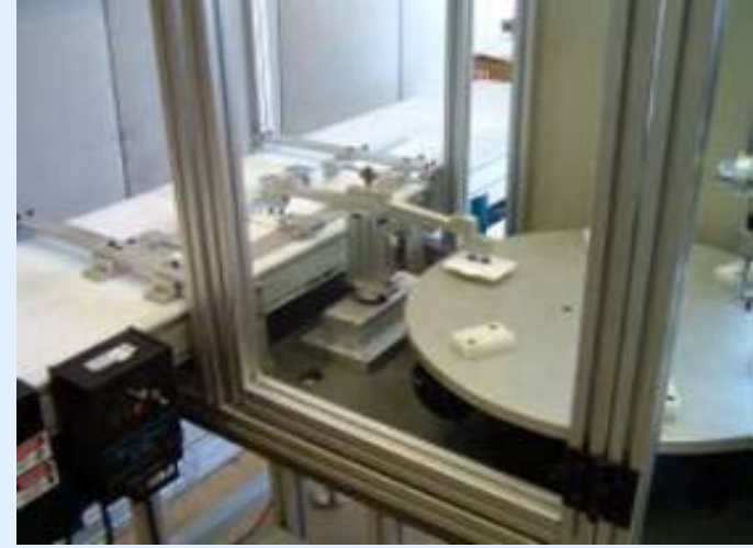
Un-attended Manufacturing cell with in-feed conveyor, part separator and auto pick and place for new and finished parts
