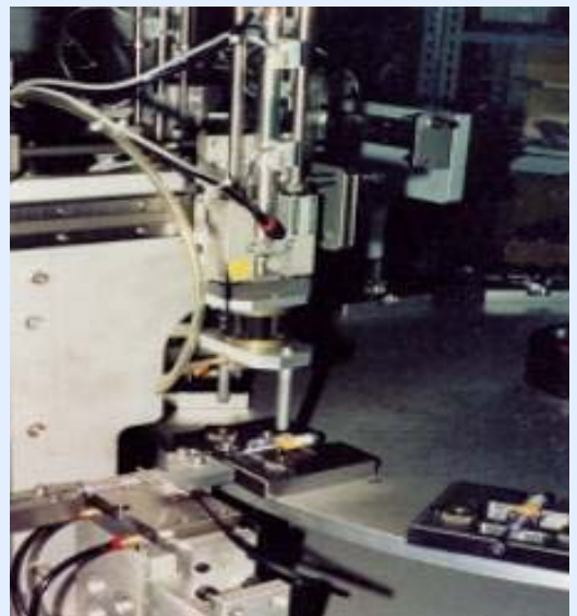
Alignment pin for accurate part insertion
