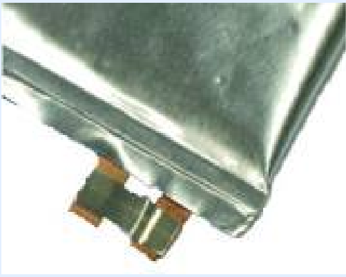
Flat battery for mobile phones - nickel to copper and aluminum
