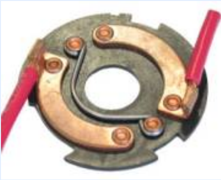
Sliding contacts -copper wire to copper contact
