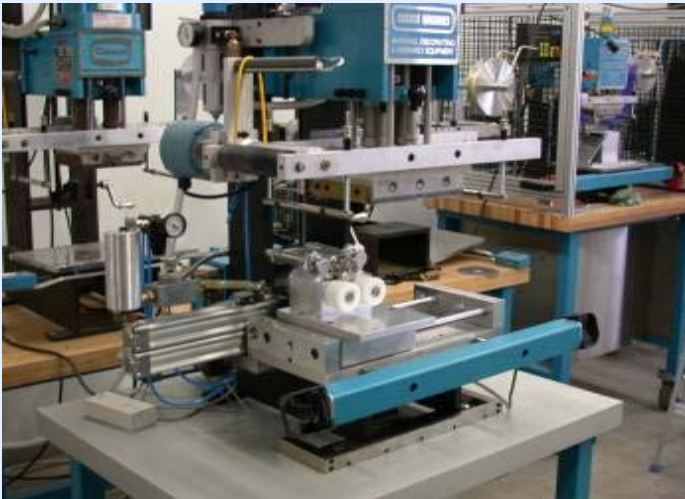
Heat Transfer System for Rotary printing up to 360° wrap around
