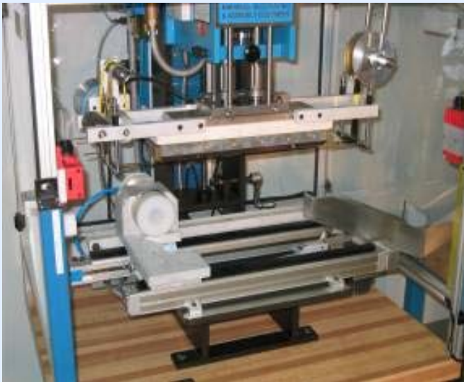
Shuttle for rotary marking (360° wrap around)
