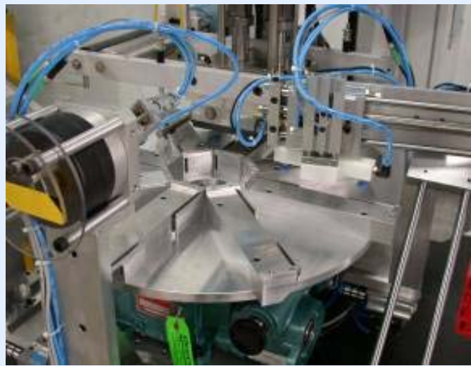
Pick & Place for automatic part loading/unloading
