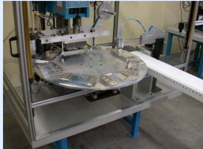
Heat Transfer on a Rotary Index Table
