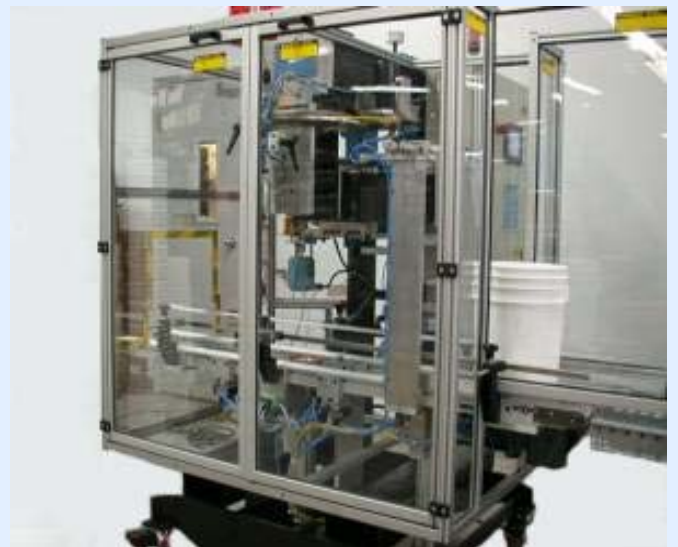
Automated hot stamping for 5 gallon bucket PE and PP material
