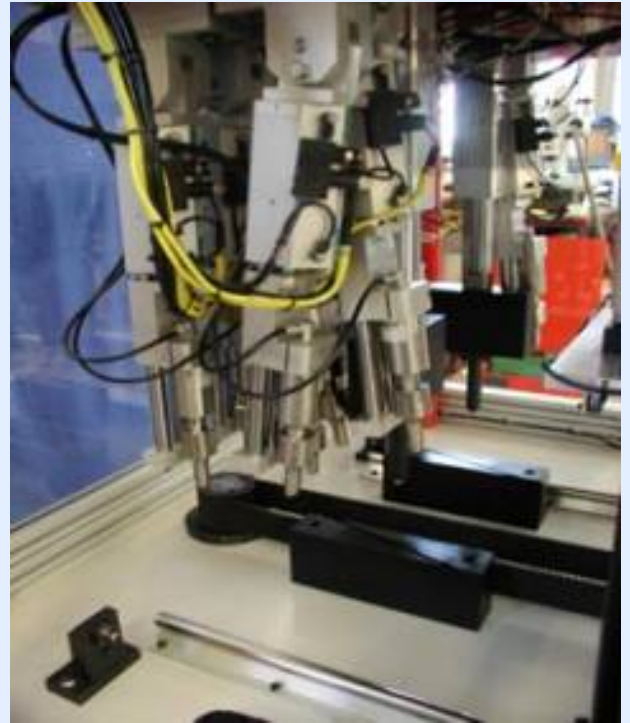
Multihead welding system for the welding of acoustic material to polypropylene moulding
